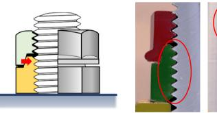
The picture shows the engagement between the threads of bolt and HLN Convex Nut.
