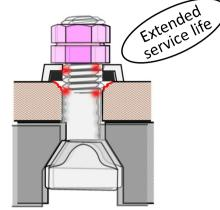
The damages act as a stress raiser applying unwanted force to the bolt shaft, which involves higher possibility of bolt breakage as the nut loosens. The function of HARDLOCK Nut to prevent rotational loosening can aid less bolt breakage.
