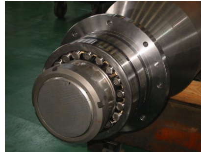
HLB (HARDLOCK Bearing Nut) M190 SS400
