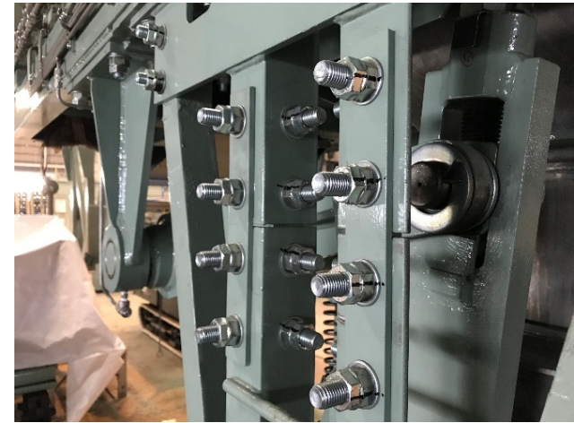
Coal Charging Car HLN M8~M33 SS400, SUS304
